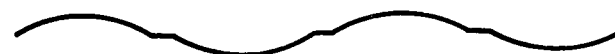
Fig. 15B — Smaller Amplitude Sine Wave with Same Amount (higher %) of Crossover (notch) Distortion.
